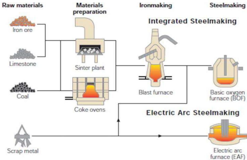
Figure 6: Process of steel making through either of these methods
