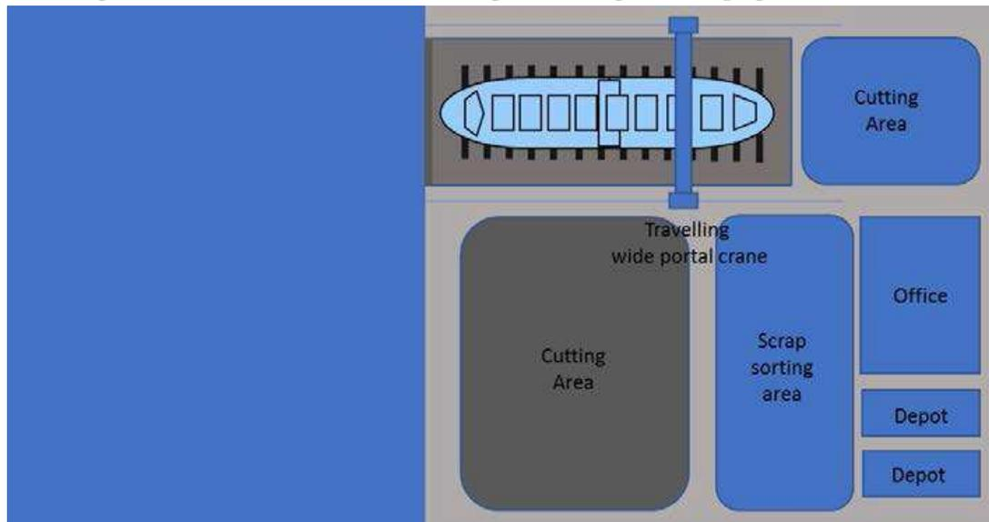
Figure 5: Layout of the dry dock method
