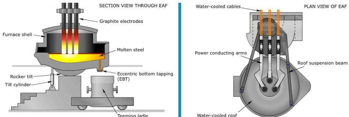
**Figure 7: Plan view of Electric Arc Furnace**
