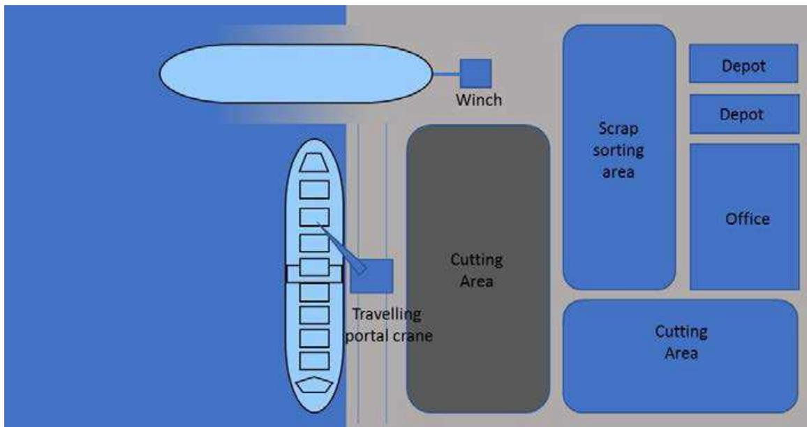
**Figure 2: Pier breaking + slipway method**
