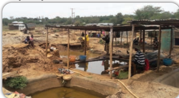
Ponds where gold is mixed with mercury. Mercury is a poisonous substance with high impacts to both human beings and environment.
