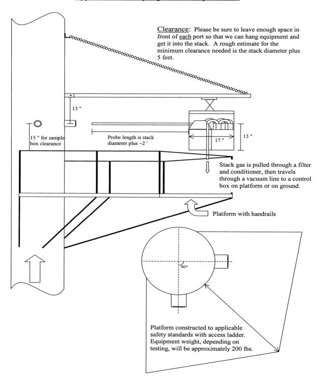
Figure 4: Typical Stack Sampling Access Requirements
