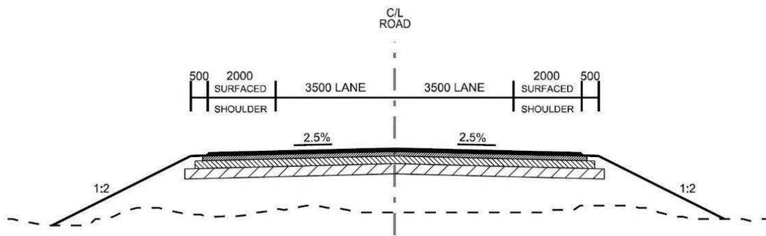
**Figure 2:** Road cross section and elevation
