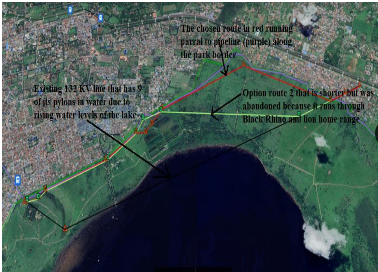
A Superimposed google earth map image showing the different power line route options
