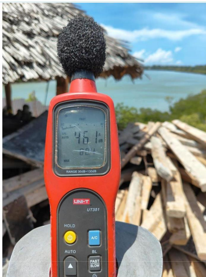
Ongoing diurnal acoustic level measurements at the proposed boundaries (source: Fieldwork May, 2025)
