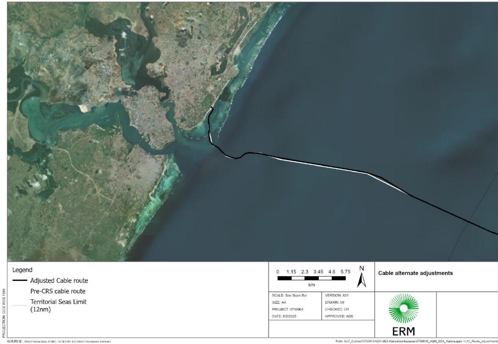
FIGURE 4-2 THE SUBSEA CABLE ALTERNATIVE ADJUSTMENTS IN THE KENYAN TERRITORIAL SEAS
