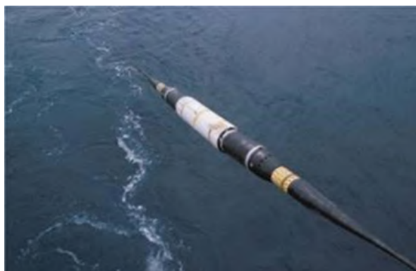
FIGURE 3-8 EXAMPLE OF A REPEATER AND FIBRE OPTIC CABLE
