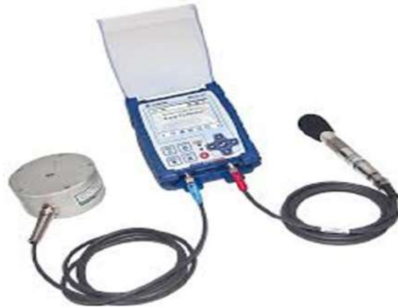
Figure 23: Ground vibration monitoring equipment
