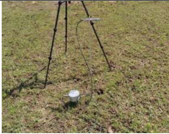
Figure 29: Vibration measurement at the proposed Kisumu Station
