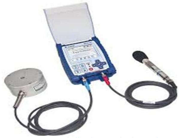
Figure 30: Ground vibration monitoring equipment
