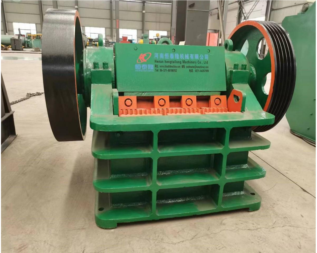
Figure 2. 3: Digital image of the secondary jaw crusher from the manufacturer (Henan Fantianliang Machinery & Equipment Co., Ltd)
