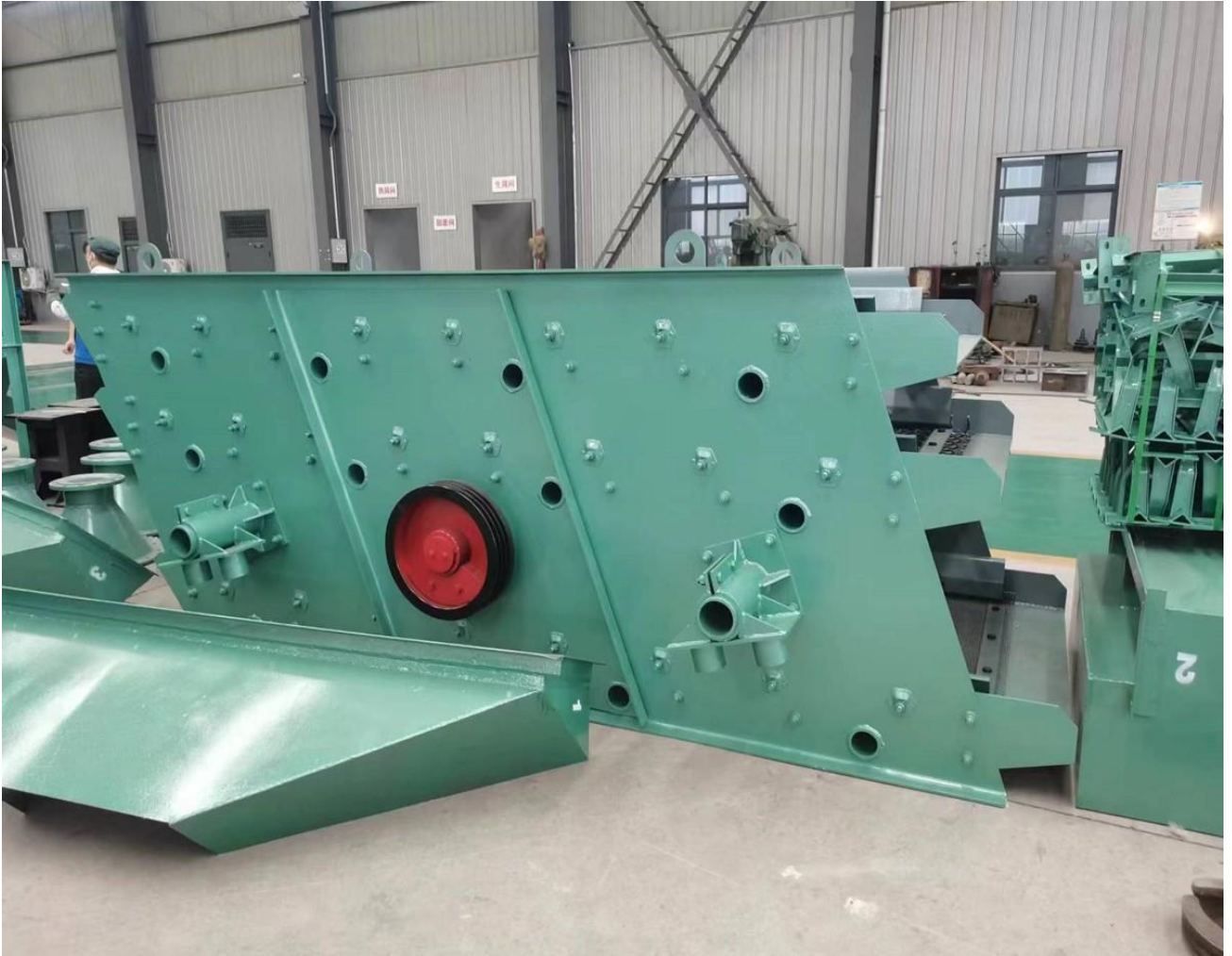
Figure 2. 4 Digital image of the vibratory screen from the manufacturer (Henan Fantianliang Machinery & Equipment Co., Ltd)
