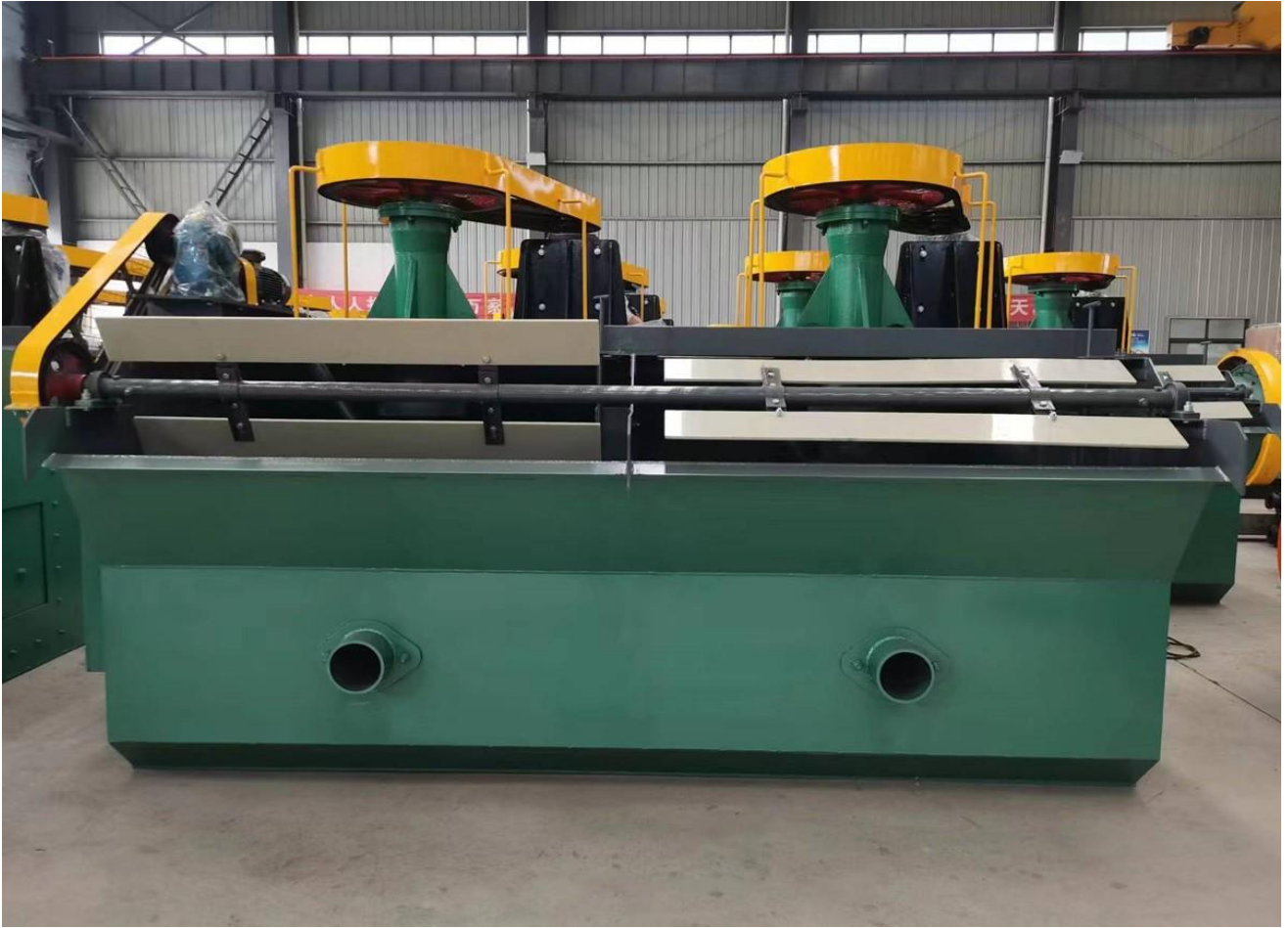
Figure 2. 7: Digital image of the flotation cells from the manufacturer (Henan Fantianliang Machinery & Equipment Co., Ltd)
