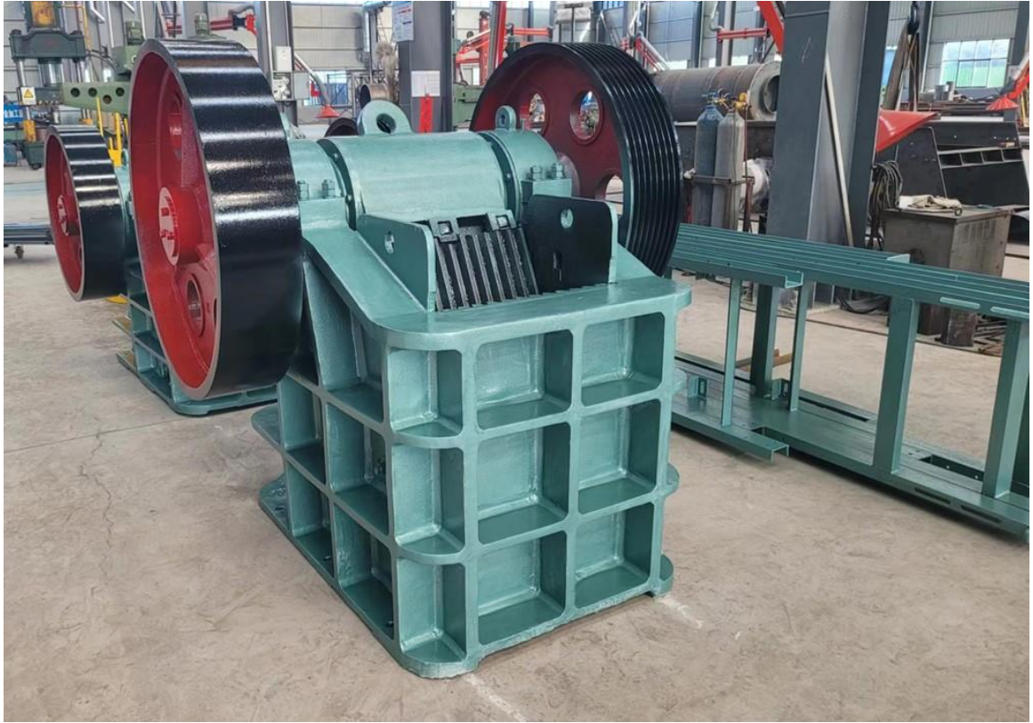
Figure 2. 2: Digital image of the primary jaw crusher from the manufacturer (Henan Fantianliang Machinery & Equipment Co., Ltd)
