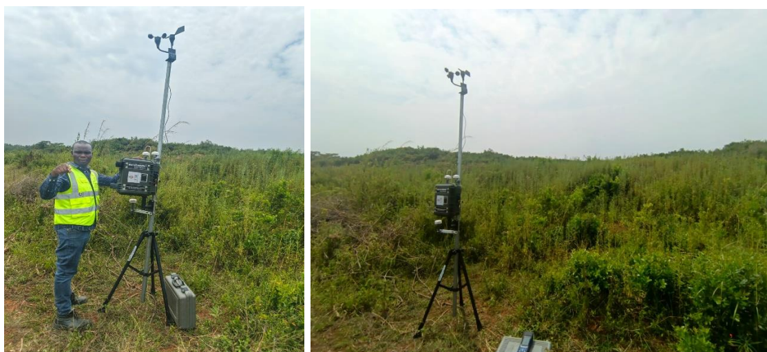
Figure 3.4.3: Ongoing determination of the ambient air quality levels at the proposed Kipenzi Sugar factory site using HAZ-SCANNER instrument
