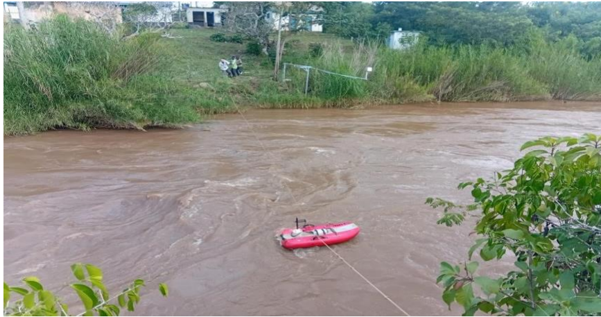
Figure 3.2.6.1: Boat gauging at River Yala (proposed abstraction point) (source: Hydrological assessment of Kipenzi sugar Ltd)
