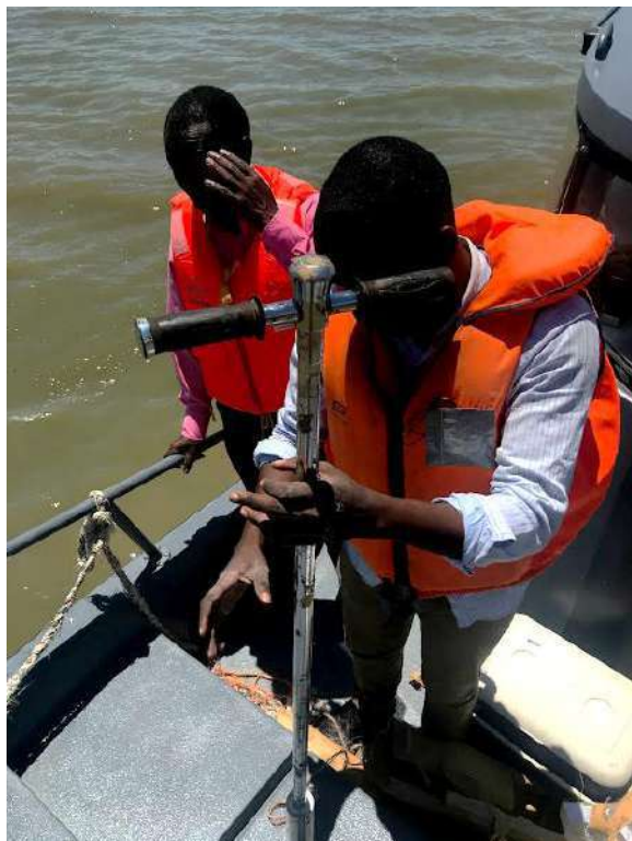
Figure 1. The Auger Sampler used in collection of sediments at River Kisat Estuary and the MRCC project site (Source: Site visits, June 2024).
