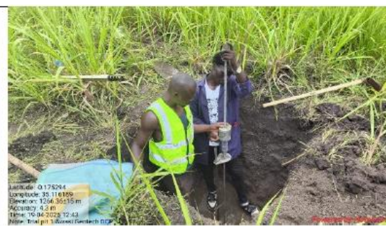
DCP Test on Trial Pit 1
